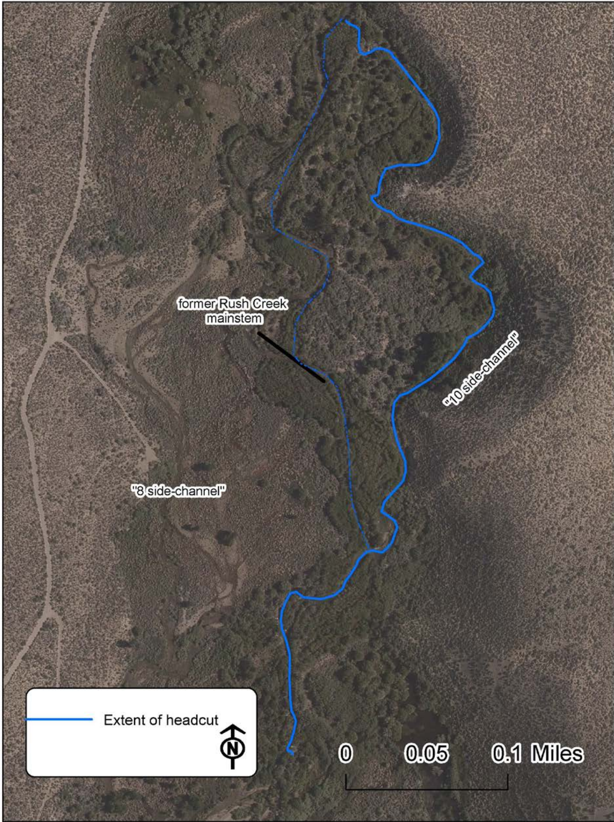
Figure 7. Spatial Extent of Headcut Associated with Knickpoint Migration on Rush Creek Following 2017 High Flows
